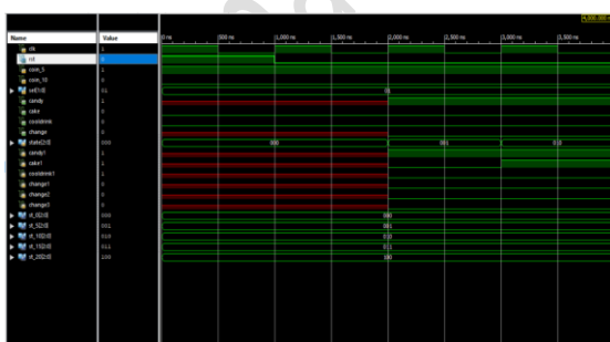
Figure-9: Simulated wave form of vending machine for candy when 5 rupee coin insert
