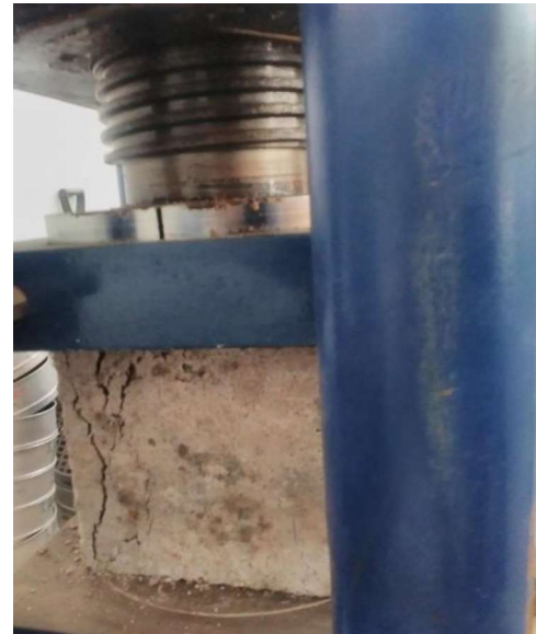
Fig. Cube testing under Compressive strength
