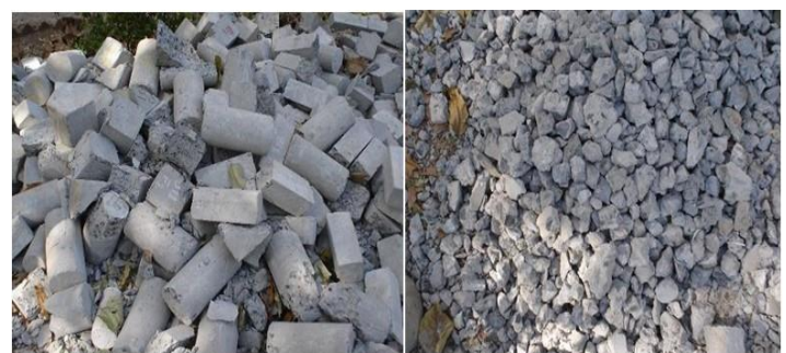
Figure 5. 1 Unprocessed Recycled coarse aggregate
