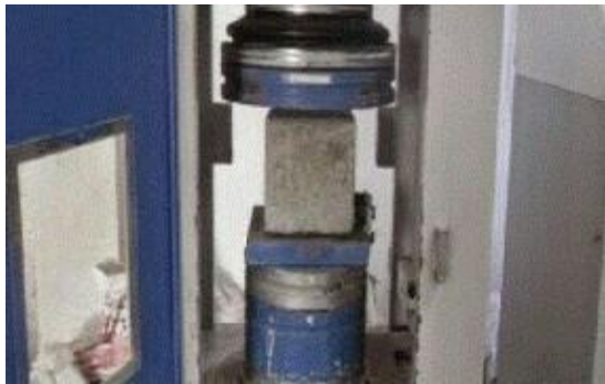
Fig 2: compressive strength testing machine
