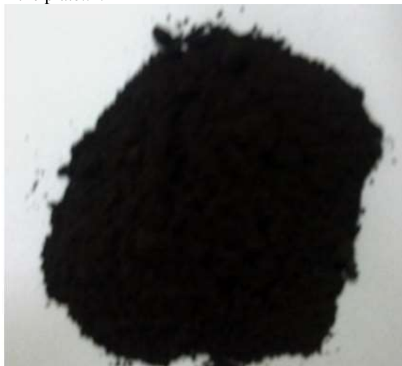
Fig 3 Photographic view of CuO nanoparticles The distribution of CuO nanoparticles at Nano scale can be observed under a Scanning electron microscope (SEM). The SEM images of CuO nanoparticles at 1 μm magnifications is shown in Plate.3.2(a) and SEM image of CuO nanoparticle on a 500 nm scale is shown in Plate.3.2(b). Preparation of Nanofluids is an important stage and Nanofluids are prepared in a systematic and careful manner. A stable Nanofluid with uniform particle dispersion is required and the same is used for measuring the thermo physical properties of Nanofluids.
