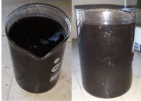
Fig :The photographic view of CuO Nano fluid suspension prepared after magnetic stirring process
